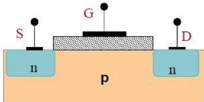
**CONSTRUCTION:** A MOSFET is a four-terminal device having source(S), gate (G), drain (D) and body (B) terminals. In general, The body of the MOSFET is in connection with the source terminal thus forming a three-terminal device such as a field-effect transistor. MOSFET is generally considered as a transistor and employed in both the analog and digital circuits
