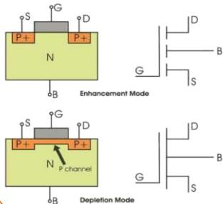
The drain and source are heavily doped p+ region and the substrate is in n-type. The current flows due to the flow of positively charged holes, and that's why known as p-channel MOSFET.
