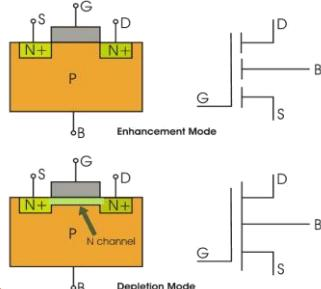
The drain and source are heavily doped N+ region and the substrate is p-type. The current flows due to the flow of negatively charged electrons and that's why known as n-channel MOSFET.
