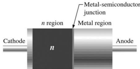
**CONSTRUCTION:** Schottky Diodes are made up of a metal electrode attached to an N-type semiconductor. Schottky diodes have no depletion layer and are classified as unipolar devices..
