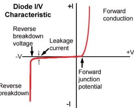
However, the reverse leakage current ( $I_R$ ) of a Schottky diode is often substantially higher than that of a PN-junction diode.
